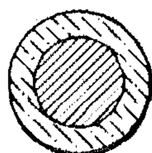
METAL NANOPARTICLE COVERED WITH UC m NANOSHELL
