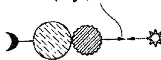
PA MOLECULE BOUND TO EEC (ATTACHED TO PLASMONICS METAL NANOPARTICLE) NANOPARTICLE BY DETACHABLE BIOCHEMICAL BOND
