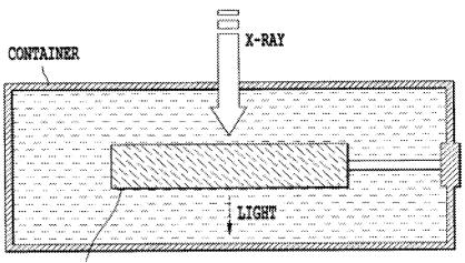
PROBE HAVING MATERIAL CONTAINING X-RAY ENERGY CONVERTER
