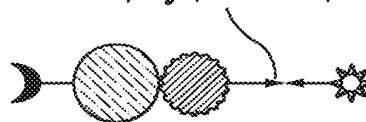
PA MOLECULE BOUND TO EEC (ATTACHED TO PLASMONICS METAL NANOPARTICLE) NANOPARTICLE BY DETACHABLE BIOCHEMICAL BOND
